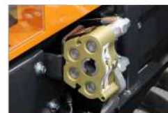
Innesti rapidi idraulici CE3N CE3N quick hydraulic couplings
